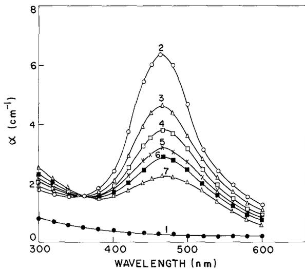
Figure 2 Optical absorption characteristics of NaCl crystals X-ray irradiated ( $1\frac{1}{2}$  h) at  $40^\circ\text{C}$  and later excited with laser light for different times. (1) as-cut NaCl; (2) X-ray at  $40^\circ\text{C}$ ; (3) (2) + 1 min laser; (4) (2) + 2 min laser; (5) (2) + 5 min laser; (6) (2) + 10 min laser; (7) (2) + 20 min laser.
