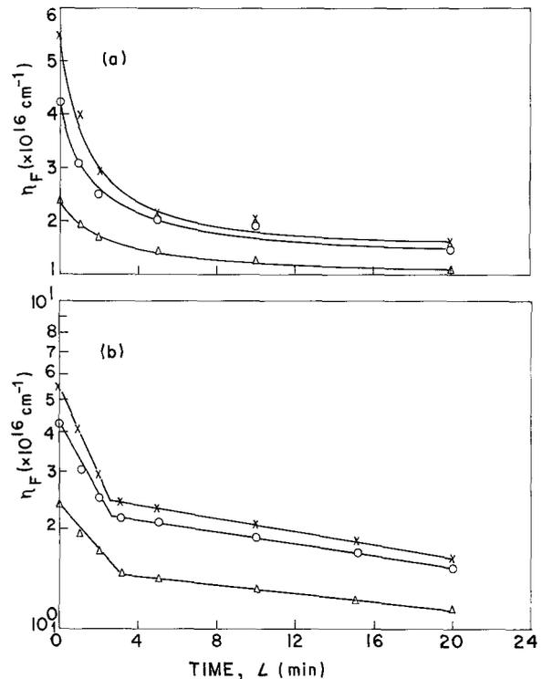
Figure 4 (a) Concentration of F-centres ( $n_F$ ) in NaCl crystals X-ray irradiated at different temperatures as a function of time of laser excitation; (b)  $\log n_F$  against time of laser excitation. ( $\times$ )  $25^\circ\text{C}$ ; ( $\circ$ )  $40^\circ\text{C}$ ; ( $\Delta$ )  $90^\circ\text{C}$ .
