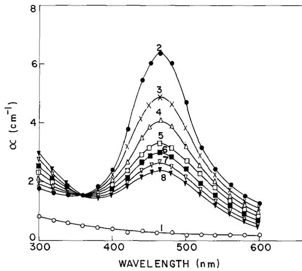
Figure 1 Optical absorption characteristics of NaCl crystals X-ray irradiated ( $1\frac{1}{2}$  h) at  $40^\circ\text{C}$  and later subjected to different a.c. fields. (1) as-cut NaCl; (2) X-ray at  $40^\circ\text{C}$ ; (3) (2) +  $1\text{ kV cm}^{-1}$ ; (4) (2) +  $2\text{ kV cm}^{-1}$ ; (5) (2) +  $5\text{ kV cm}^{-1}$ ; (6) (2) +  $10\text{ kV cm}^{-1}$ ; (7) (2) +  $15\text{ kV cm}^{-1}$ ; (8) (2) +  $20\text{ kV cm}^{-1}$ .
