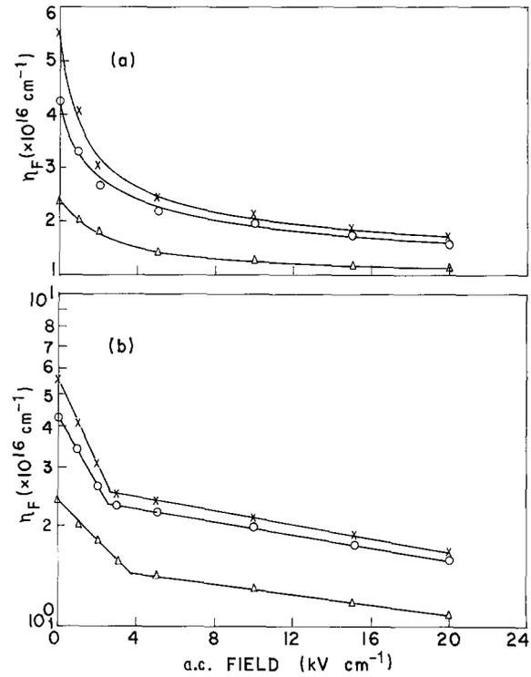
Figure 3 (a) Concentration of F-centres ( $n_F$ ) in NaCl crystals X-ray irradiated at different temperatures as a function of a.c. field; (b)  $\log n_F$  against a.c. field. ( $\times$ )  $25^\circ\text{C}$ ; ( $\circ$ )  $40^\circ\text{C}$ ; ( $\Delta$ )  $90^\circ\text{C}$ .
