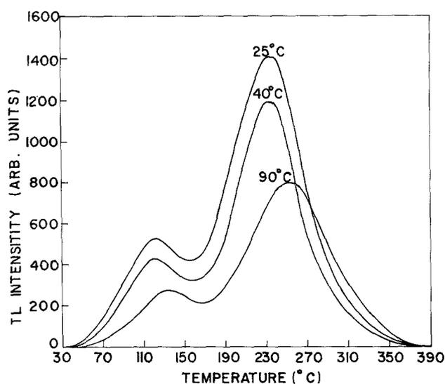
Figure 5 Thermoluminescence characteristics of NaCl crystals X-ray irradiated at different temperatures.
